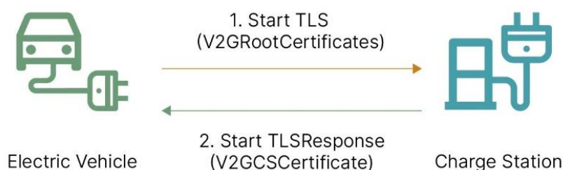
Figure 2-3: Initial TLS handshake authorisation of certificates for PnC
